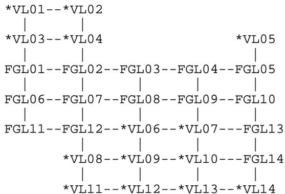
Assuming that the FGL TRILL switches in this campus all implement Step (A), then end stations connected through a VL port can be connected anywhere in the campus to VL or FGL TRILL switches and, if in the same VLAN, will communicate. End stations connected through an FGL port on FGL TRILL switches will communicate if their local VLANs are mapped to the same FGL.
