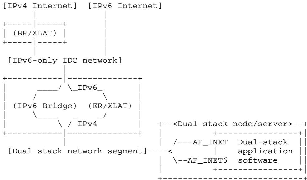
Figure 4: A Network-Based Edge Relay Containing an IPv6 Bridge
