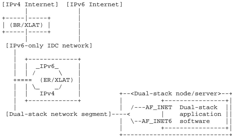
Figure 3: A Network-Based Edge Relay "on a Stick"
