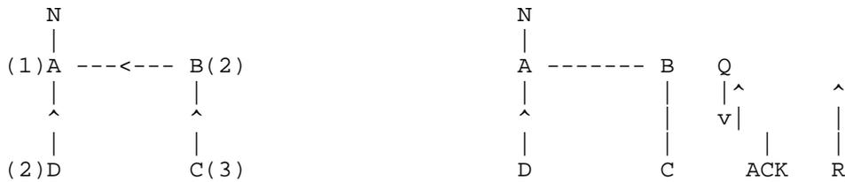
Figure 4: No Feasible Successors When Link between A and B Fails
