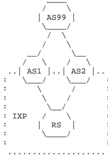
Figure 3: BGP NEXT\_HOP Hijacking Using a Route Server
