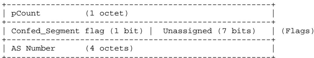
Figure 5: `Secure_Path Segment` Format
