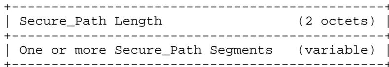
Figure 4: `Secure_Path` Format
