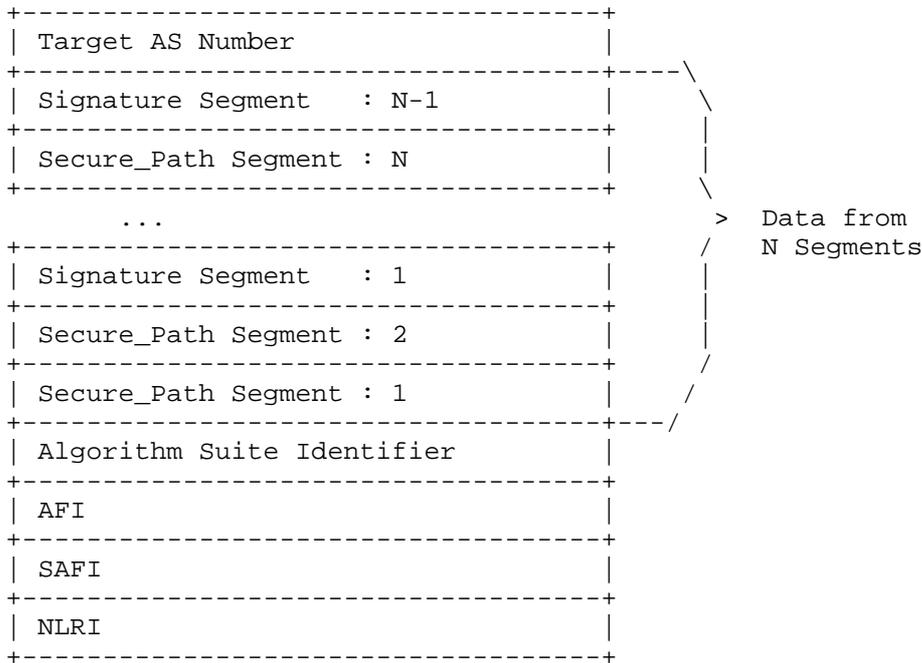
Figure 9: Sequence of Octets to Be Hashed for Signature Verification of Signature Segment N;  $N = 1, 2, \dots, K$ , Where K Is the Number of AS Hops in the BGPsec\_PATH Attribute
