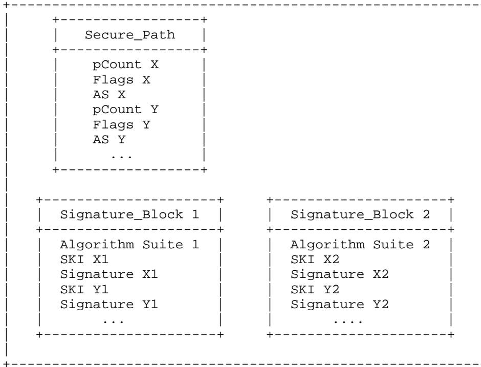
Figure 2: High-Level Diagram of the BGPsec\_PATH Attribute
