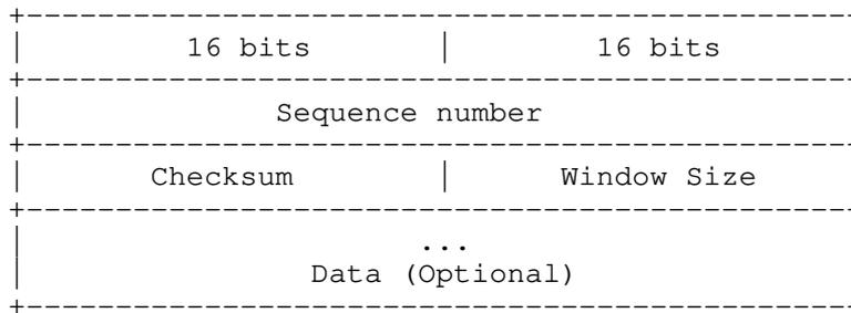
Figure 6: Transport Protocol Data Packet Format
