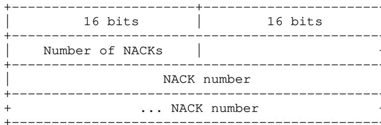
Figure 7: Transport Protocol NACK Packet Format
