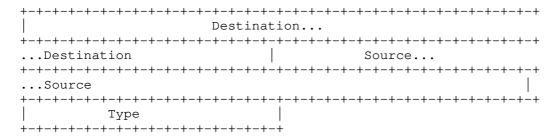
Figure 9: Ethernet II Header
