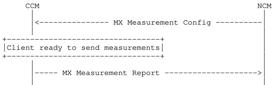
Figure 12: MAMS Client Measurement Configuration and Reporting Procedure
