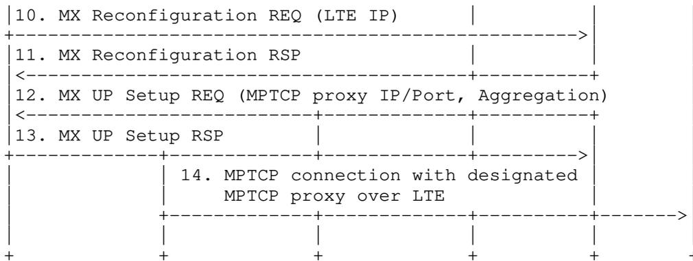
Figure 18: MAMS-Assisted MPTCP Proxy as User Plane - Initial Setup with LTE Leg
