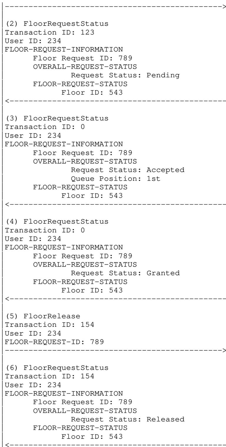
Figure 2: Requesting and releasing a floor
