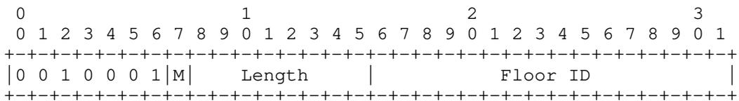
Figure 27: FLOOR-REQUEST-STATUS-HEADER format
