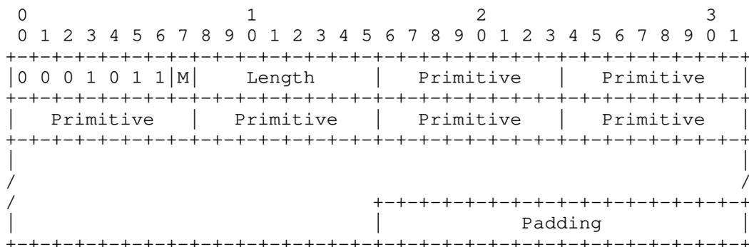
Figure 18: SUPPORTED-PRIMITIVES format
