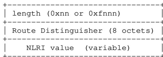
Figure 7: Flow Specification NLRI for MPLS
