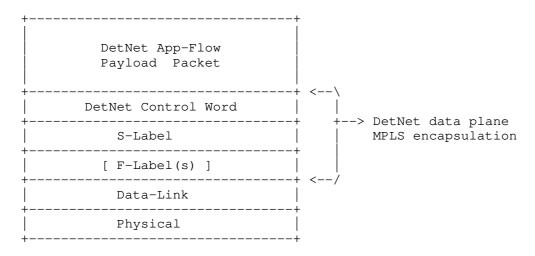
Figure 4: Encapsulation of a DetNet App-Flow in an MPLS PSN
