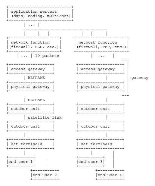
3. Use Cases for Improving SATCOM System Performance Using Network Coding
