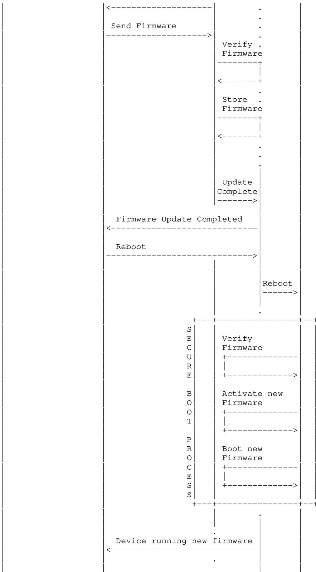
Figure 2: First Example Flow for a Firmware Update
