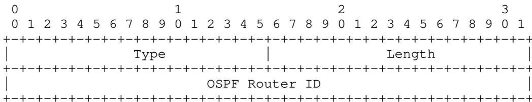
Figure 1: Prefix Source OSPF Router-ID Sub-TLV Format
