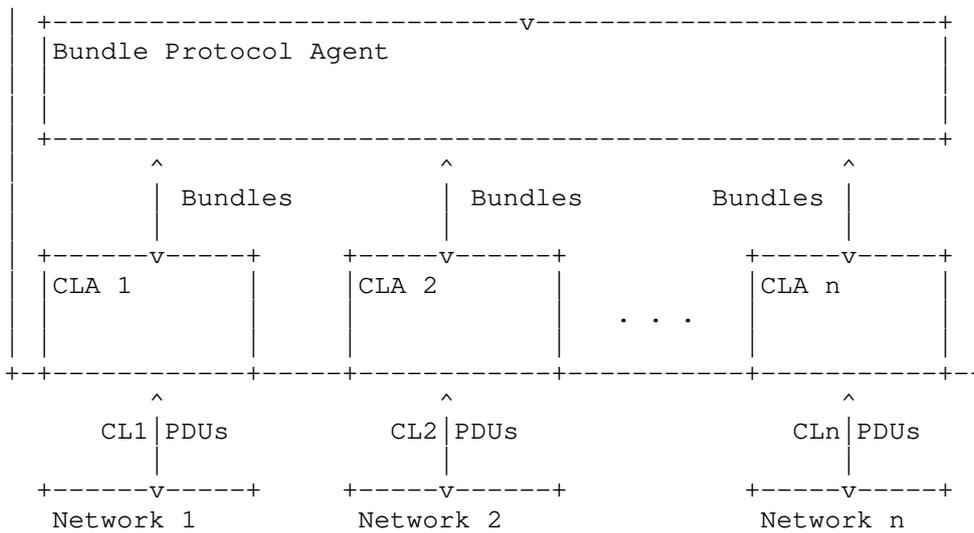
Figure 2: Components of a Bundle Node
