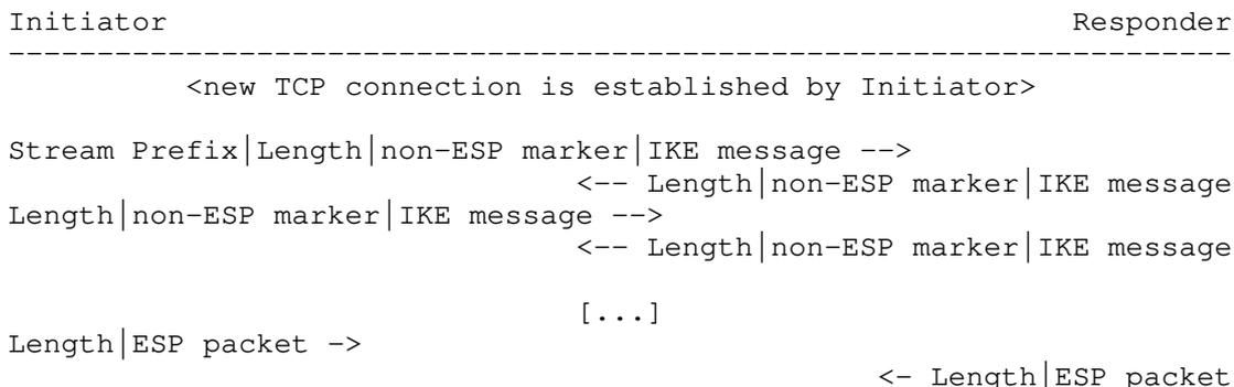
If other framing protocols are used within TCP to further encapsulate or encrypt the stream of IKE and ESP messages, the stream prefix must be at the start of the TCP Originator's IKE and ESP message stream within the added protocol layer (Appendix A). Although some framing protocols do support negotiating inner protocols, the stream prefix should always be used in order for implementations to be as generic as possible and not rely on other framing protocols on top of TCP.
