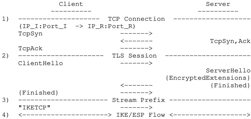
1. If a previous TCP connection was broken (for example, due to a TCP Reset), the client is responsible for re-initiating the TCP connection. The TCP Originator's address and port (IP\_I and Port\_I) may be different from the previous connection's address and port.
