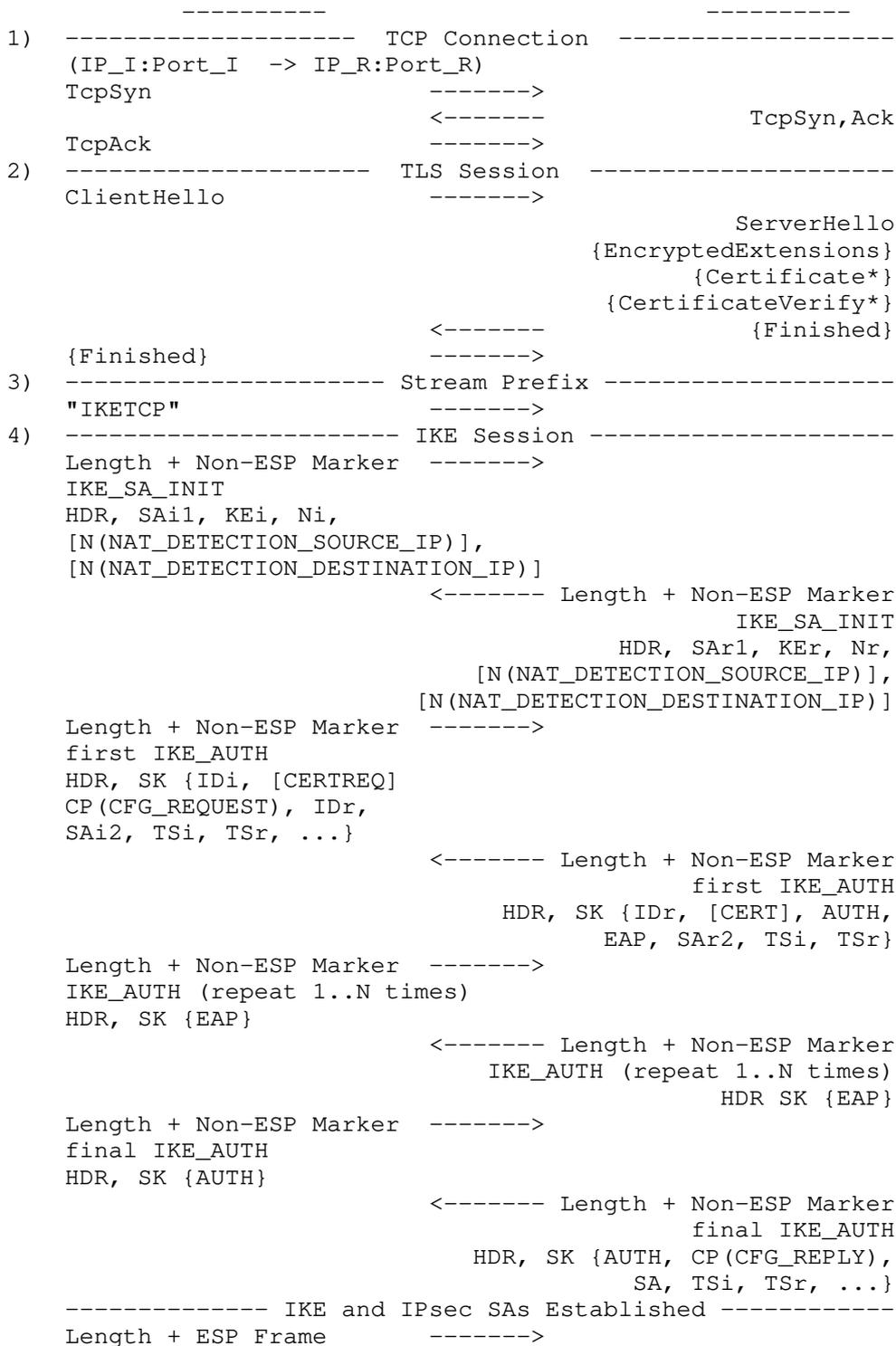
1. The client establishes a TCP connection with the server on port 4500 or on an alternate preconfigured port that the server is listening on.
